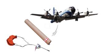
The P3 drop tube and parachute used during air deployment. Upon exiting the drop tube, the swivel wing design of the SØ allows for a seamless transition to flight.
