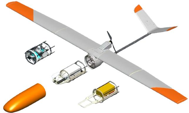
Figure 3: BST’s modular field-swappable payload system.
