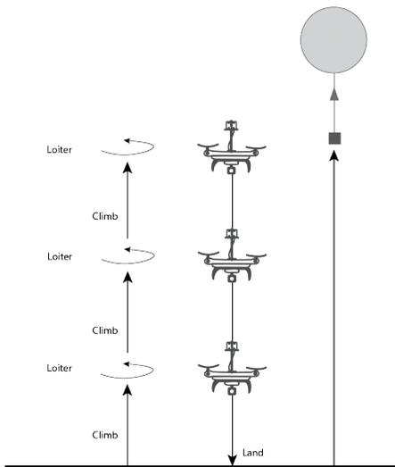
Figure 1: Vertical profiling using multi-rotor UAS or balloons.
