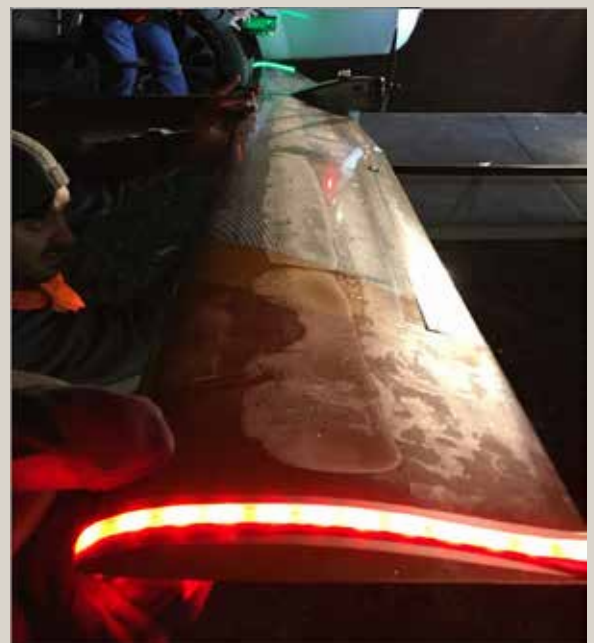
Clear ice build-up on a wing of an S2 after a high altitude test flight in the winter.
